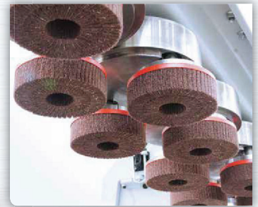
Planetary head technology for all-round edge machining with cup brushes.
